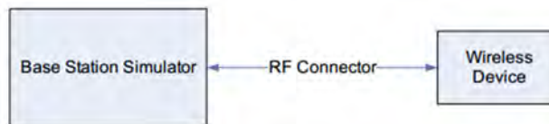
Figure 8.1 Power Measurement Setup
