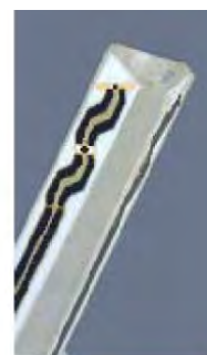
Figure E.2.2 Probe Thick-Film Technique
