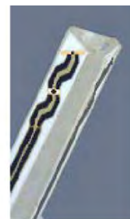
Figure 3.3 Probe Thick-Film Technique
