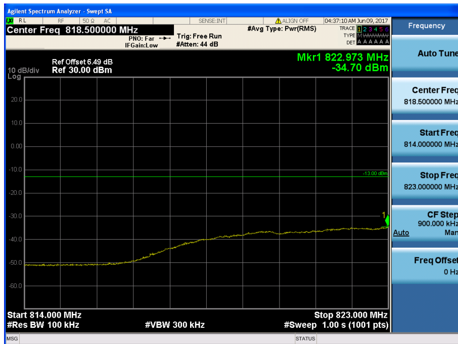
LTE Band 5 / 10MHz / 16QAM - RB Size/Offset (50/0)
