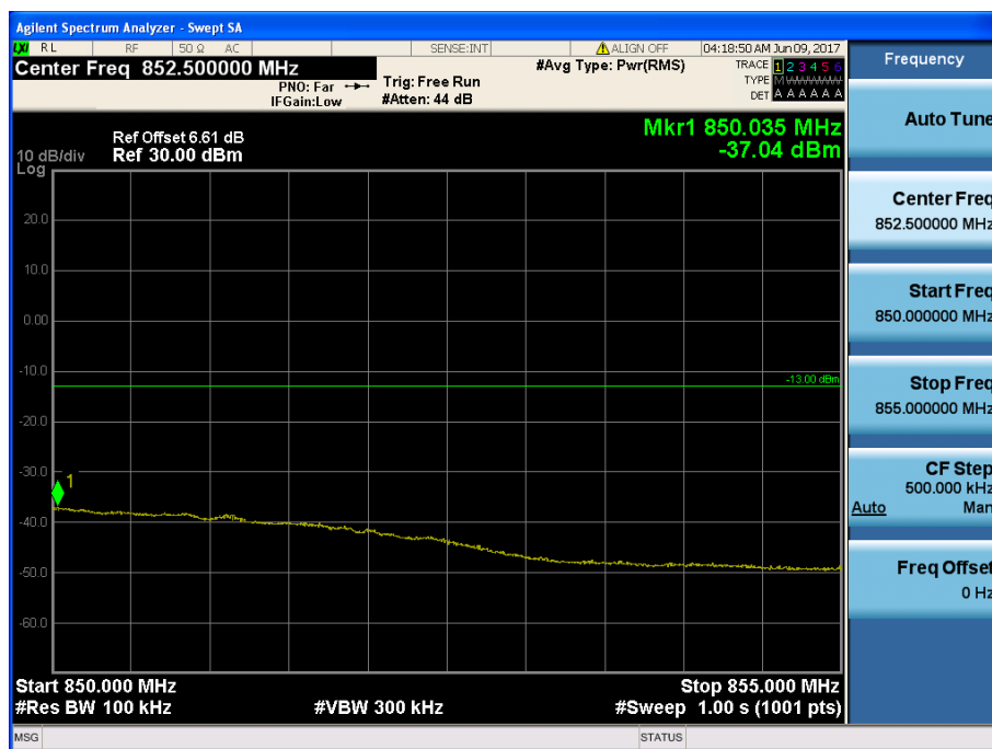
LTE Band 5 / 5MHz / 16QAM - RB Size/Offset (25/0)
