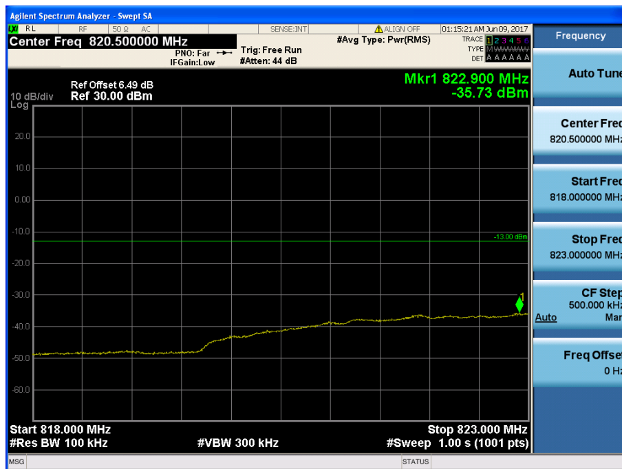
LTE Band 5 / 5MHz / QPSK Offset/Size (25/0)
