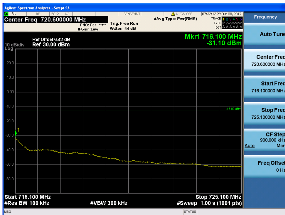
LTE Band 17 / 10MHz / QPSK - RB Size/Offset (25/25)
