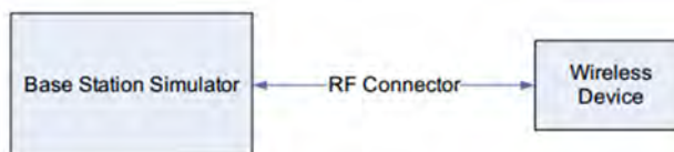
Figure 9.1 Power Measurement Setup
