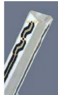
Figure 3.3 Probe Thick-Film Technique
