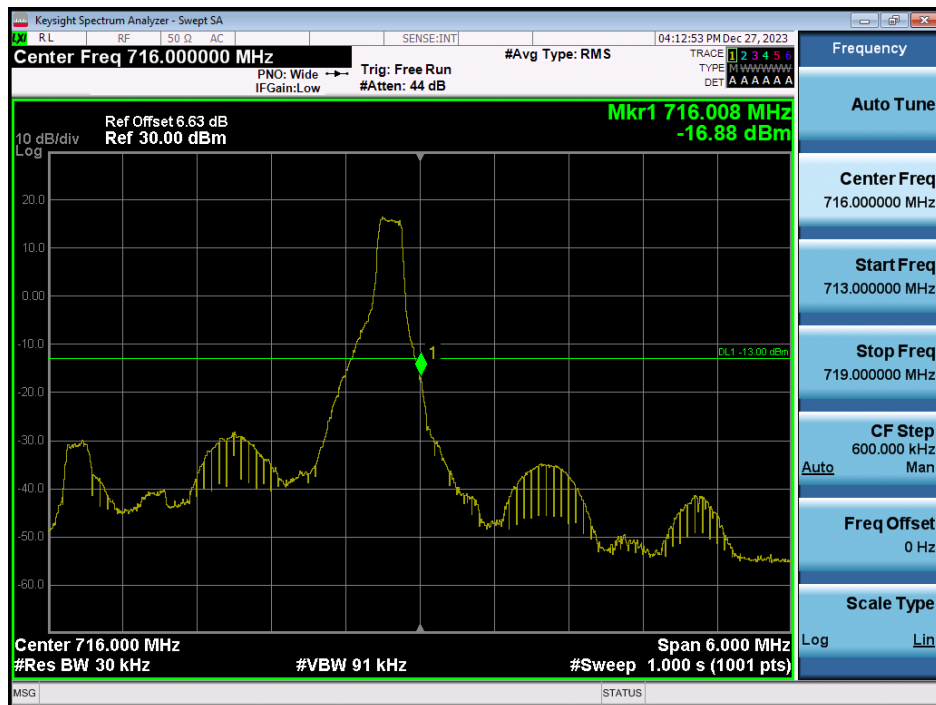
LTE Band 12 / 3MHz / 16QAM - RB Size/Offset (1/14)
