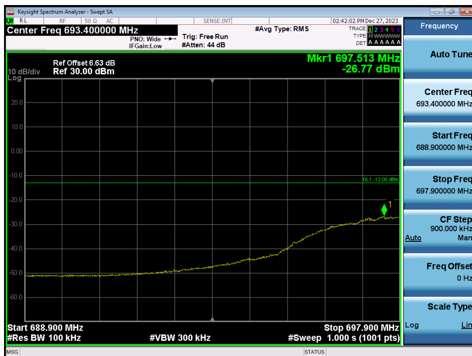
LTE Band 12 / 10MHz / QPSK - RB Size/Offset (25/0)
