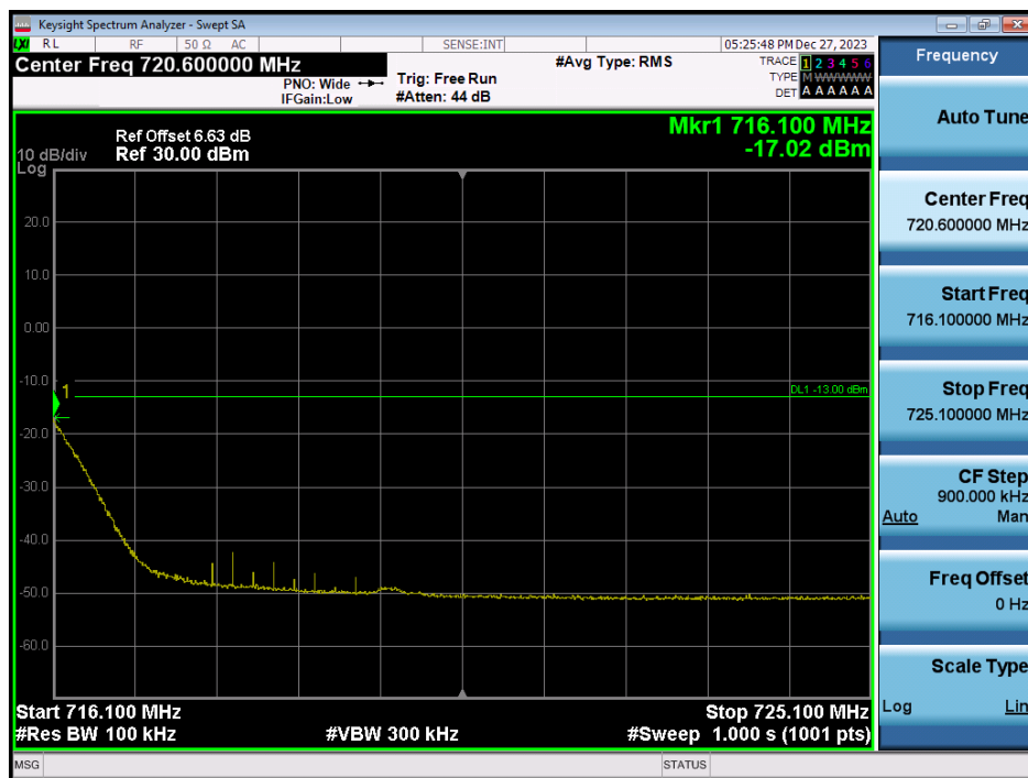
LTE Band 12 / 10MHz / 16QAM - RB Size/Offset (1/49)
