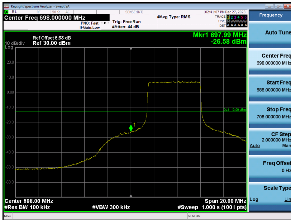
LTE Band 12 / 10MHz / QPSK - RB Size/Offset (25/0)
