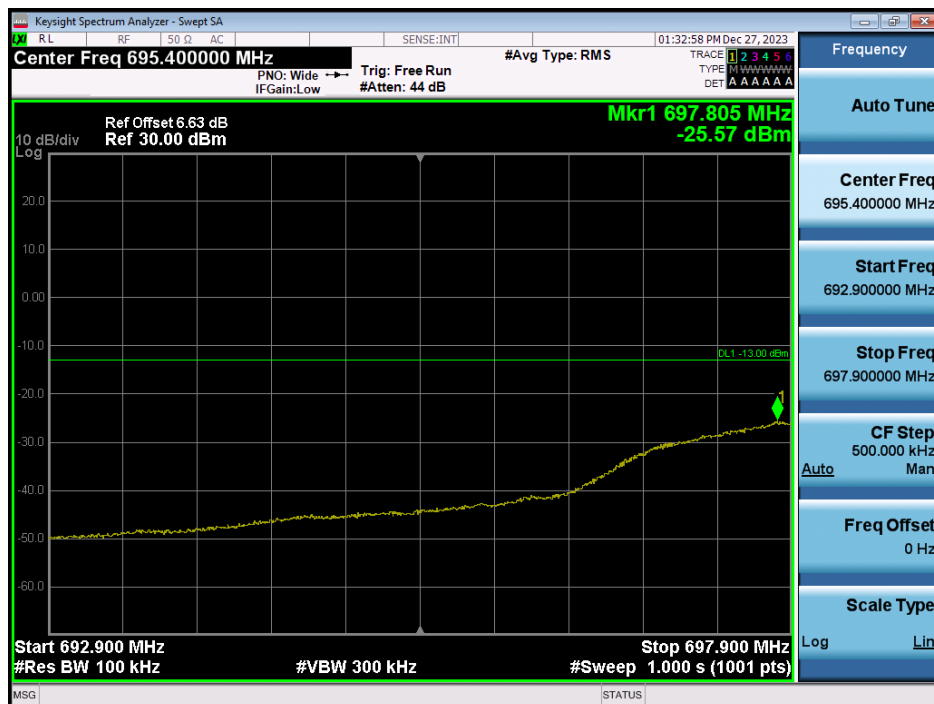
LTE Band 12 / 3MHz / QPSK - RB Size/Offset (15/0)
