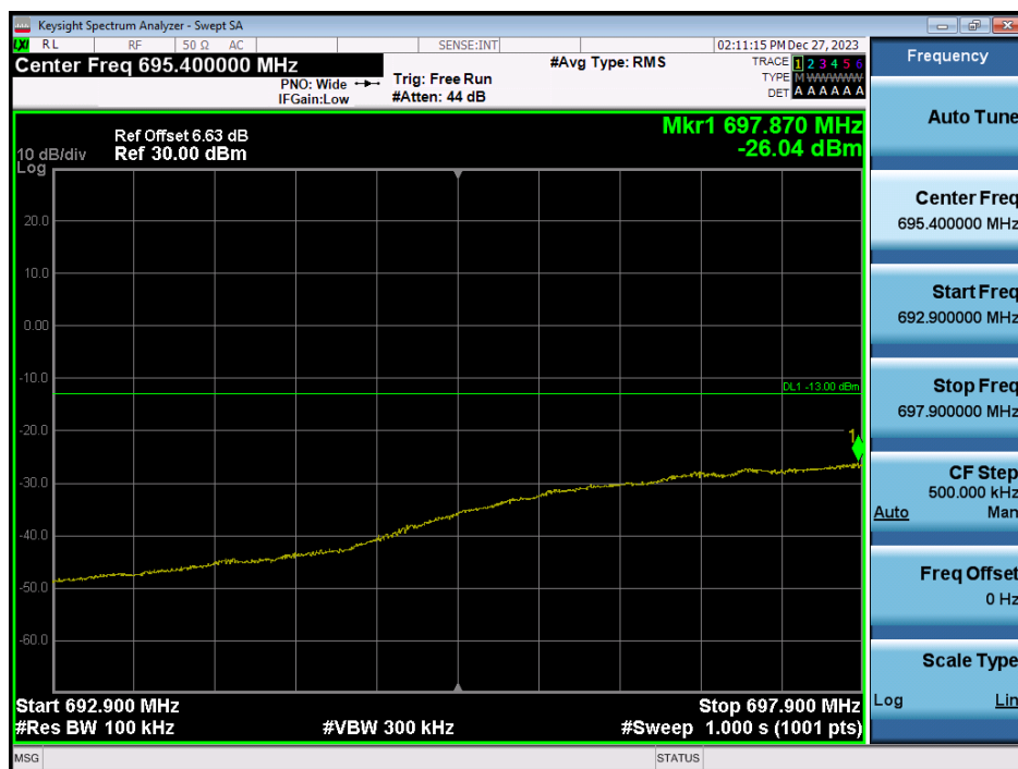
LTE Band 12 / 5MHz / QPSK - RB Size/Offset (25/0)
