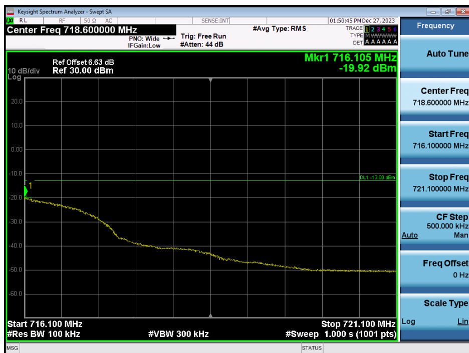
LTE Band 12 / 3MHz / QPSK - RB Size/Offset (8/7)
