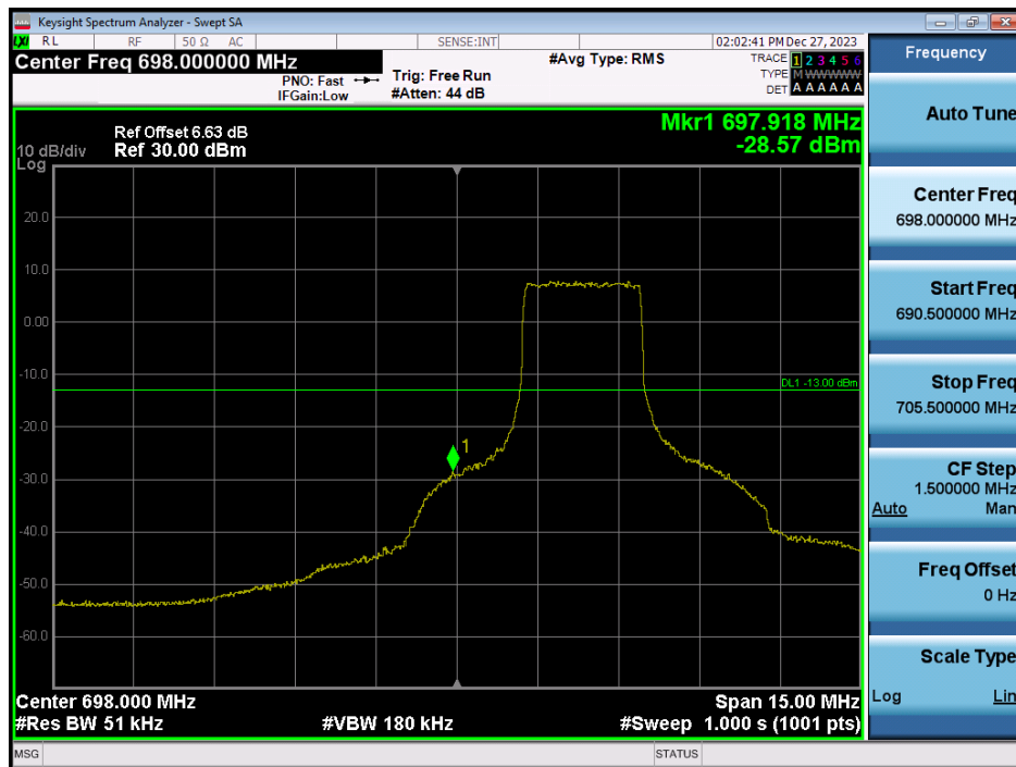
LTE Band 12 / 5MHz / QPSK - RB Size/Offset (12/0)
