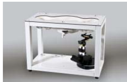
Figure E.5.1 SAM Twin Phantom
