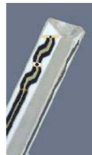
Figure E.2.2 Probe Thick-Film Technique
