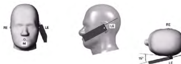
Figure 5.3 Front, Side and Top View of Ear/15° Position
