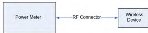
Figure 6.1.1 Power Measurement Setup
