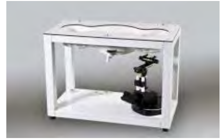
Figure E.5.1 SAM Twin Phantom
