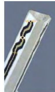
Figure E.2.2 Probe Thick-Film Technique
