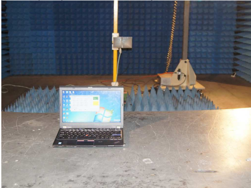
Photograph 8: Set-up for Spurious Emissions of Keyboard, 18GHz – 25GHz
