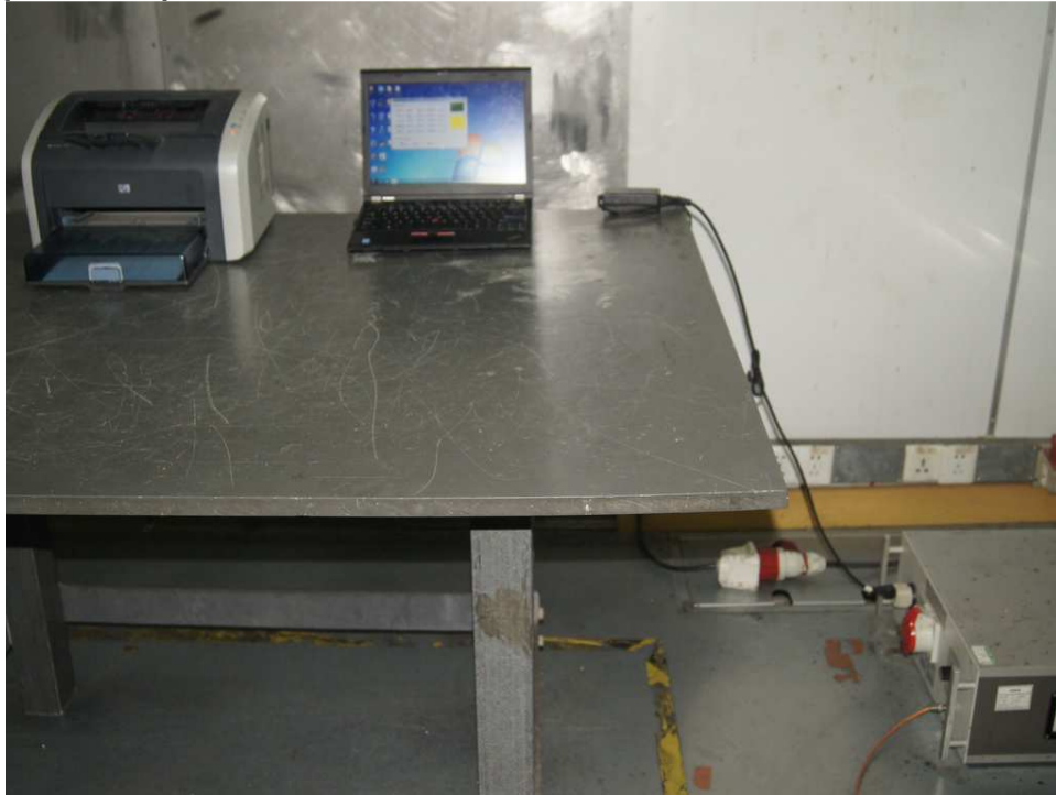
Photograph 2: Set-up for Spurious Emissions of Keyboard, below 30MHz
