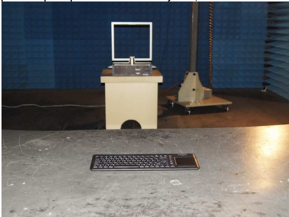
Photograph 2: Set-up for Spurious Emissions of Keyboard, below 30MHz
