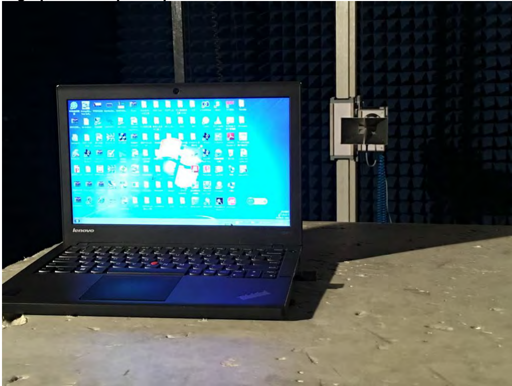
Photograph 4: Set-up for Spurious Emissions of 18 – 26.5GHz
