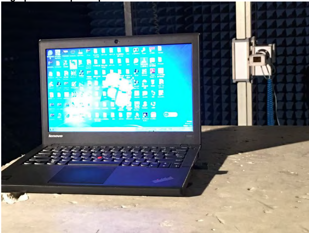
Photograph 4: Set-up for Spurious Emissions of 18 – 26.5GHz
