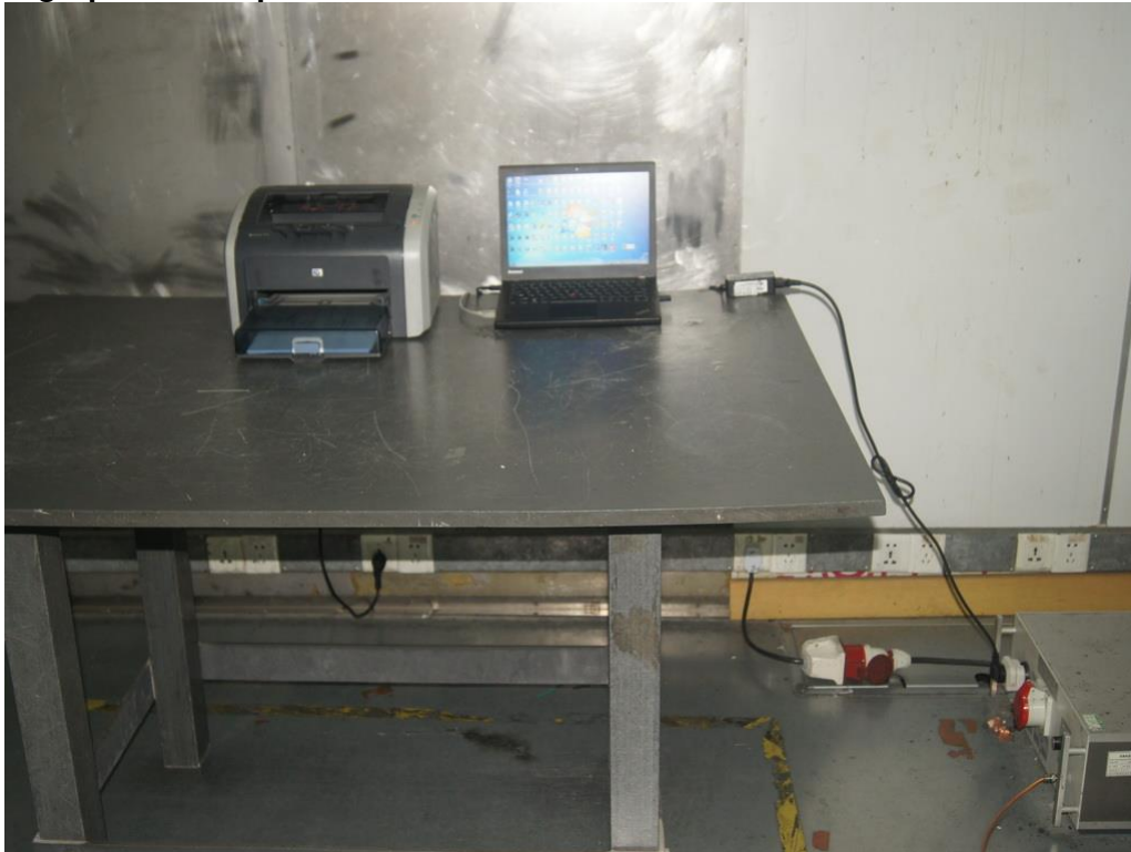
Photograph 2: Set-up for Spurious Emissions for below 1GHz
