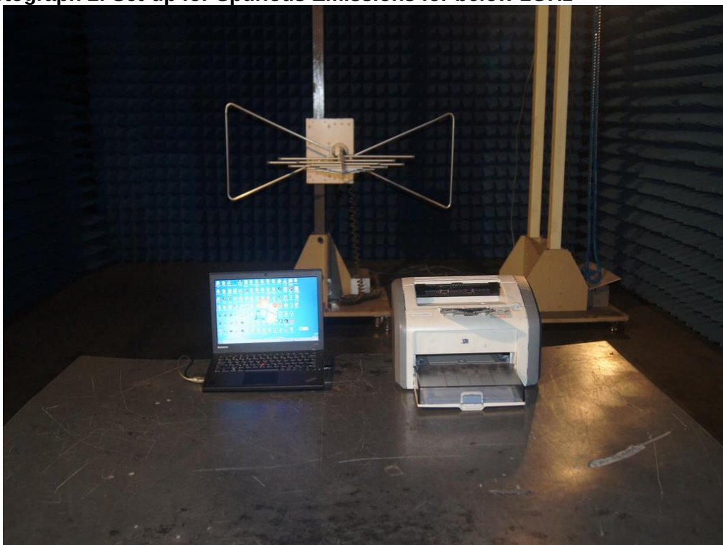
Photograph 2: Set-up for Spurious Emissions for below 1GHz
