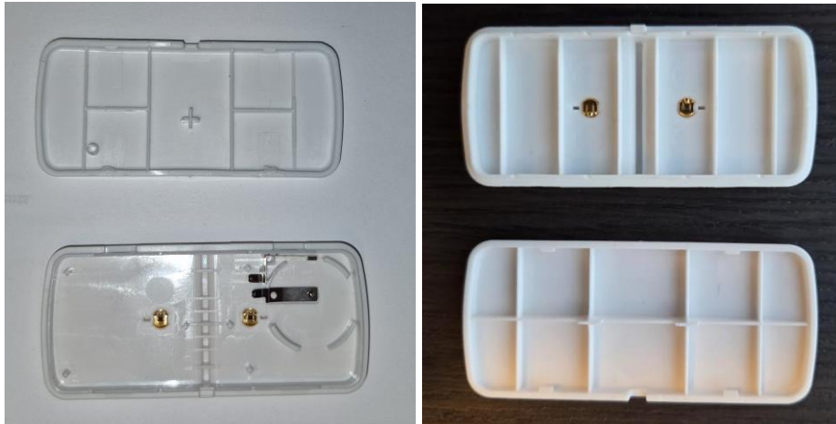
Figure 1 Nox S2 device – enclosure with stamped parts
