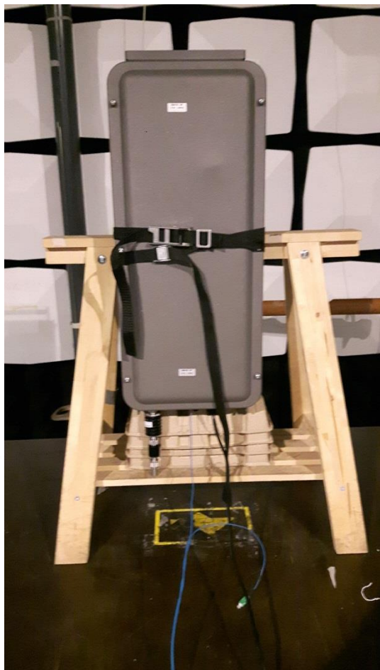
Test set up radiated emission 30 MHz – 1GHz
