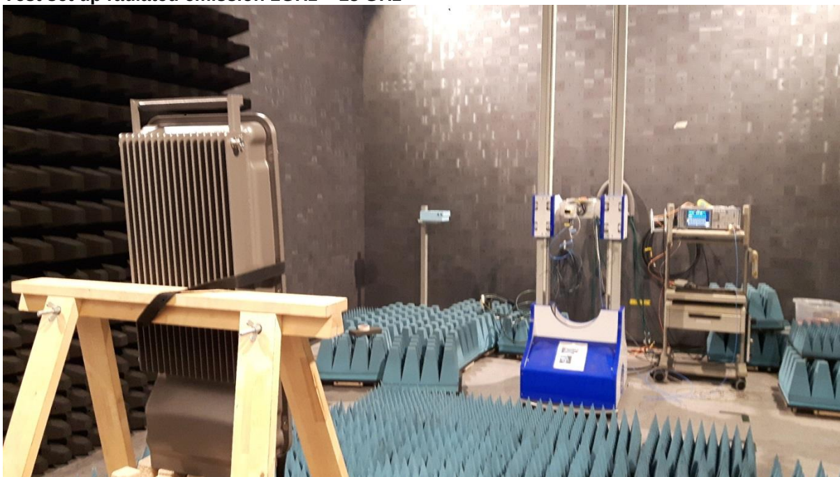
Test set up radiated emission 18 GHz – 27 GHz
