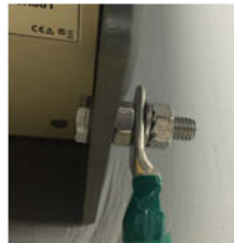
Figure 57 Remote Ground Connection
