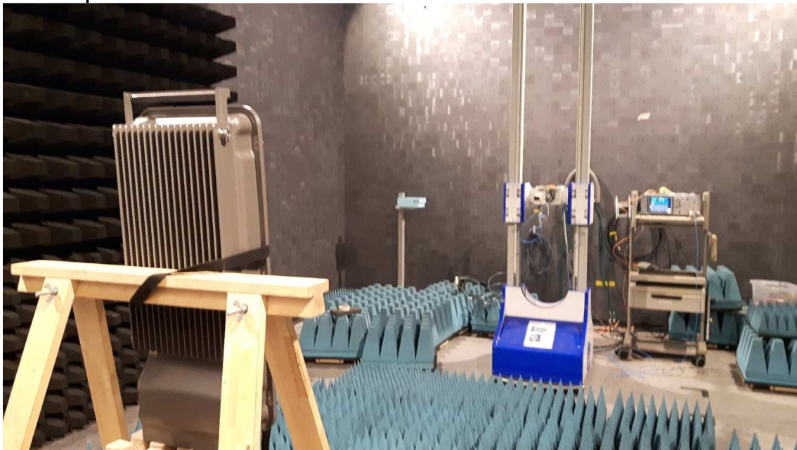
Test set up radiated emission 18 GHz – 26 GHz
