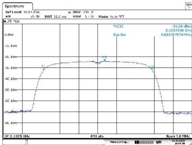
AWS Occupied bandwidth WCDMA agc on
