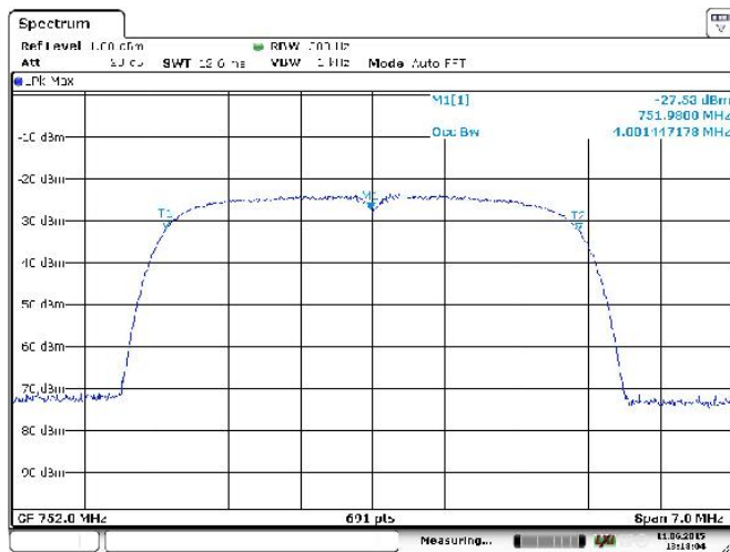
700 MHz Occupied bandwidth WCDMA agc off.
