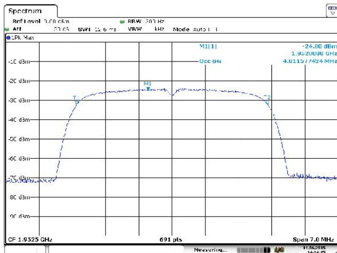
1900 MHz Occupied bandwidth WCDMA agc off
