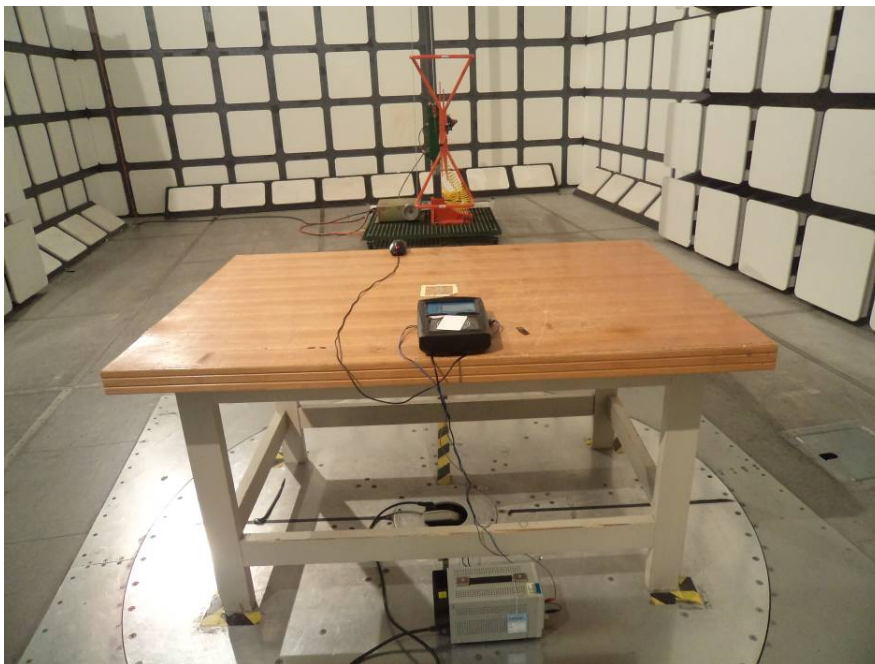
Radiated Emissions Back View (Above 30 MHz)
