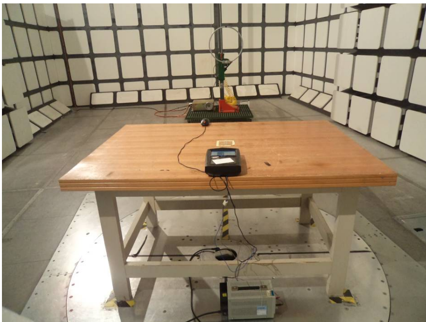
Radiated Emissions Back View (Below 30 MHz)
