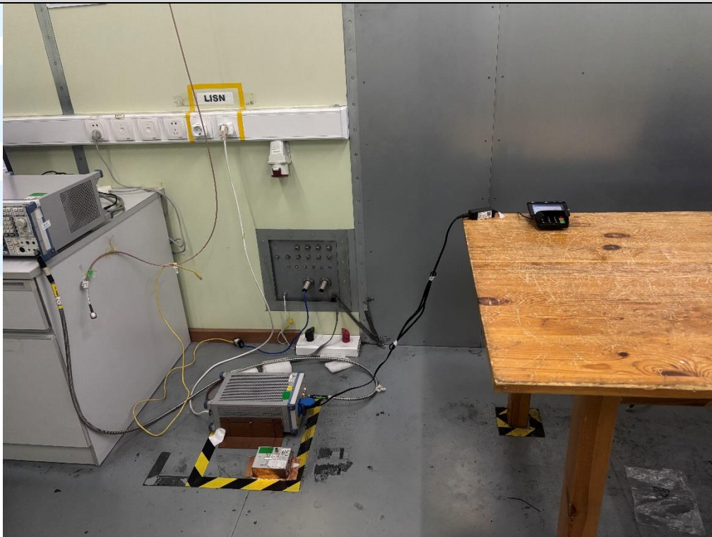
Conducted Emission Test Setup
