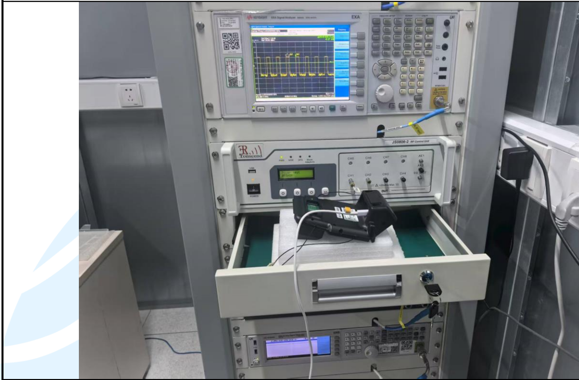
RF Conducted Test Setup
