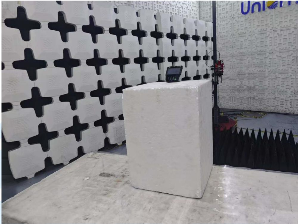
Radiated emission Test Setup (Above 1 GHz)
