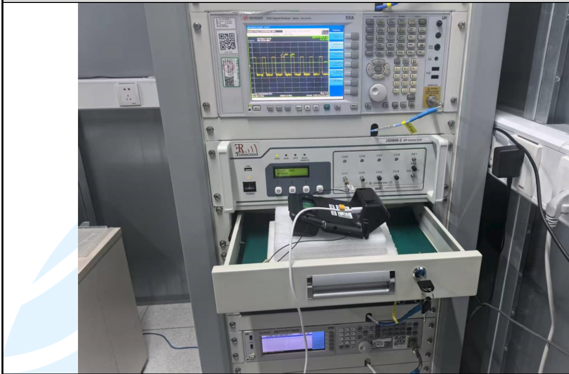
RF Conducted Test Setup
