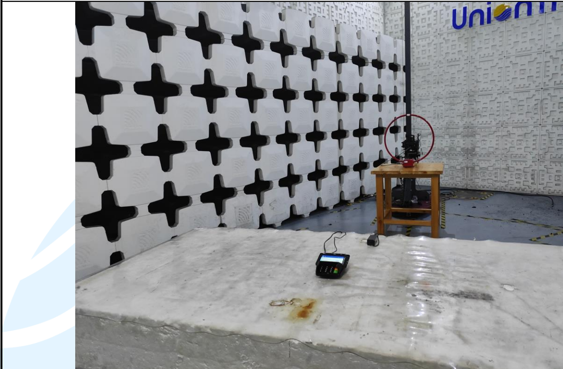
Radiated emission Test Setup (Below 30 MHz)
