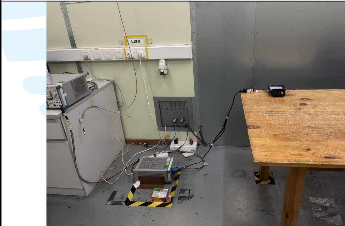
Conducted Emission Test Setup
