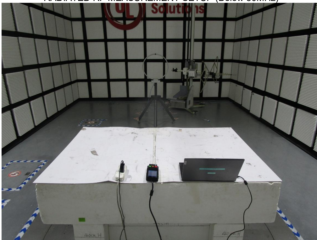
RADIATED RF MEASUREMENT SETUP (Below 30MHz)
