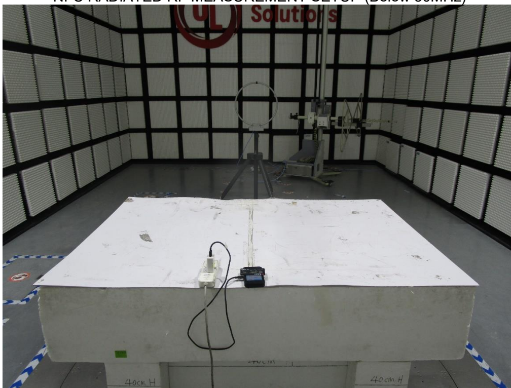
NFC RADIATED RF MEASUREMENT SETUP (Below 30MHz)
