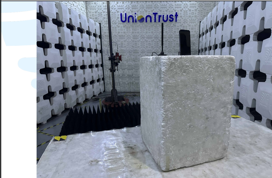
Radiated emission Test Setup (Above 1 GHz)
