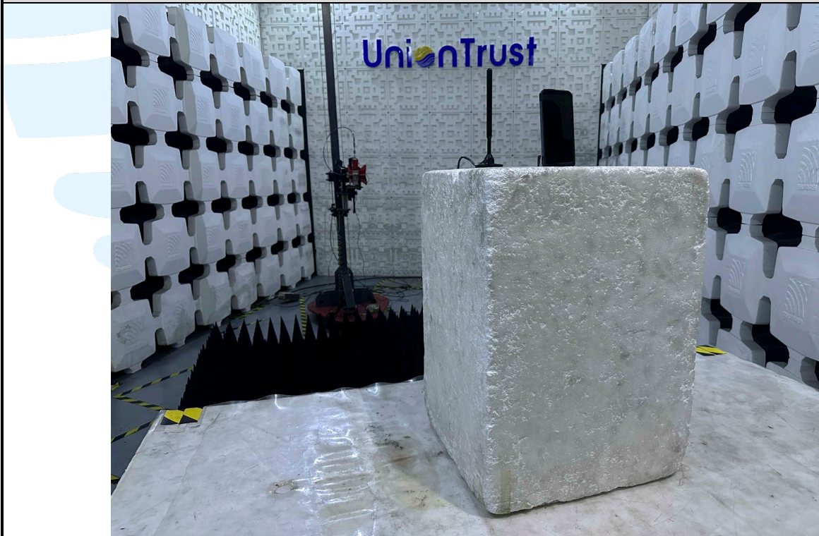
Radiated emission Test Setup (Above 1 GHz)
