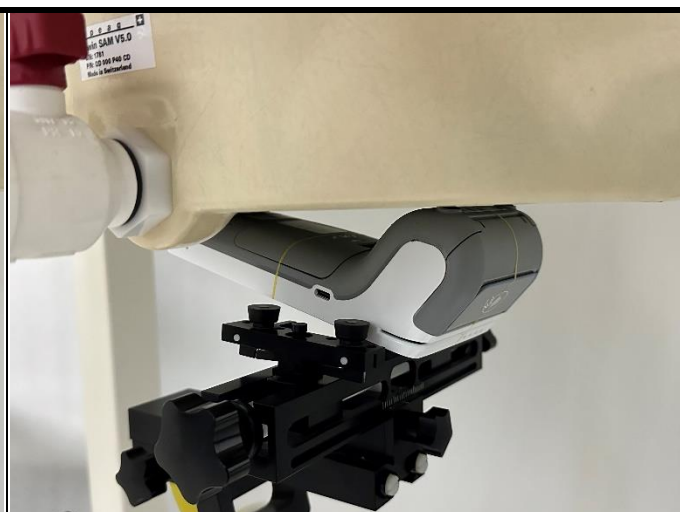
Rear Face of EUT with 0 cm Gap
