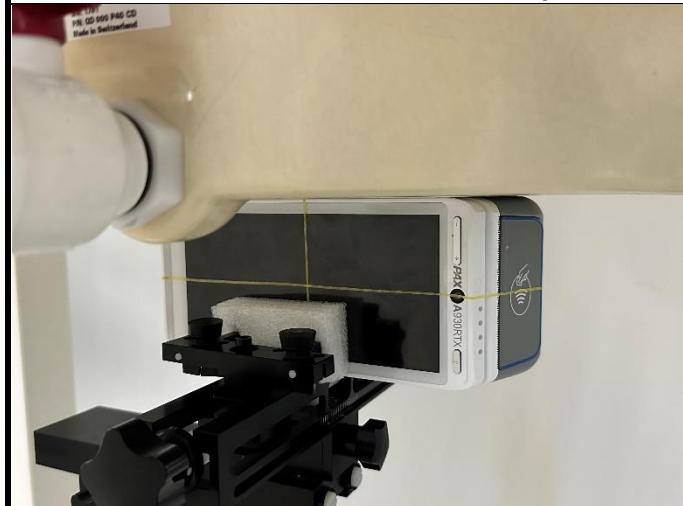
Left Side of EUT with 0 cm Gap
