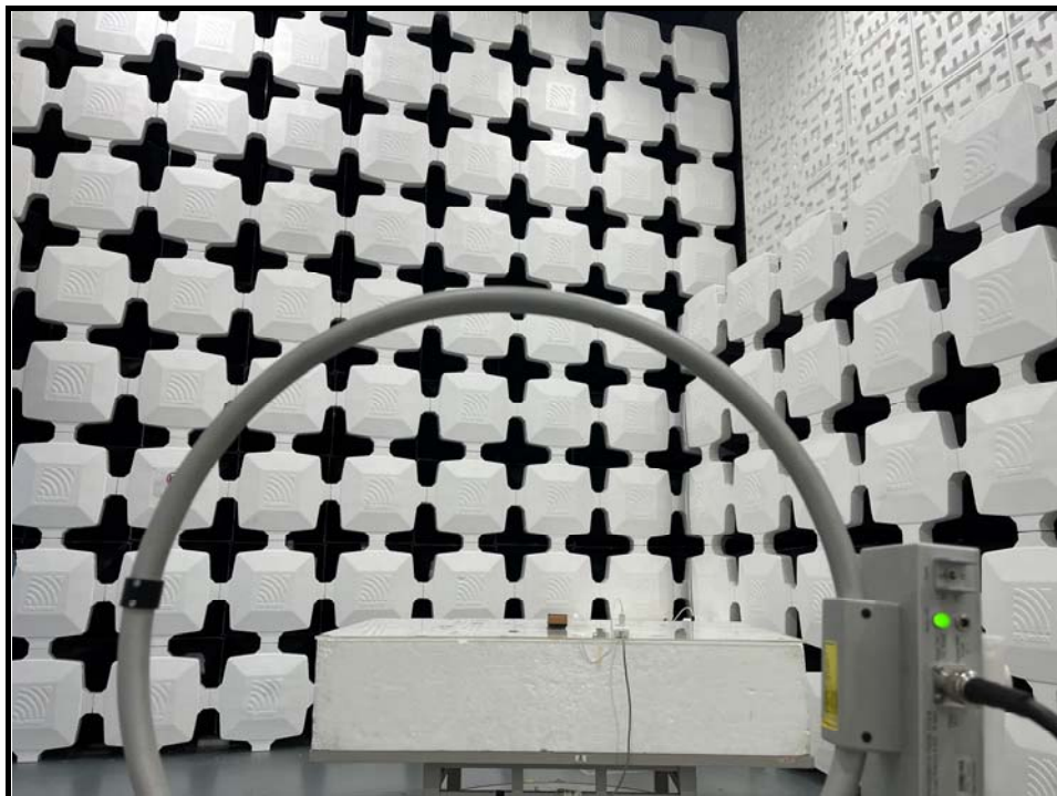
Fig. 1 Radiated emission setup photo(Below 30MHz)
