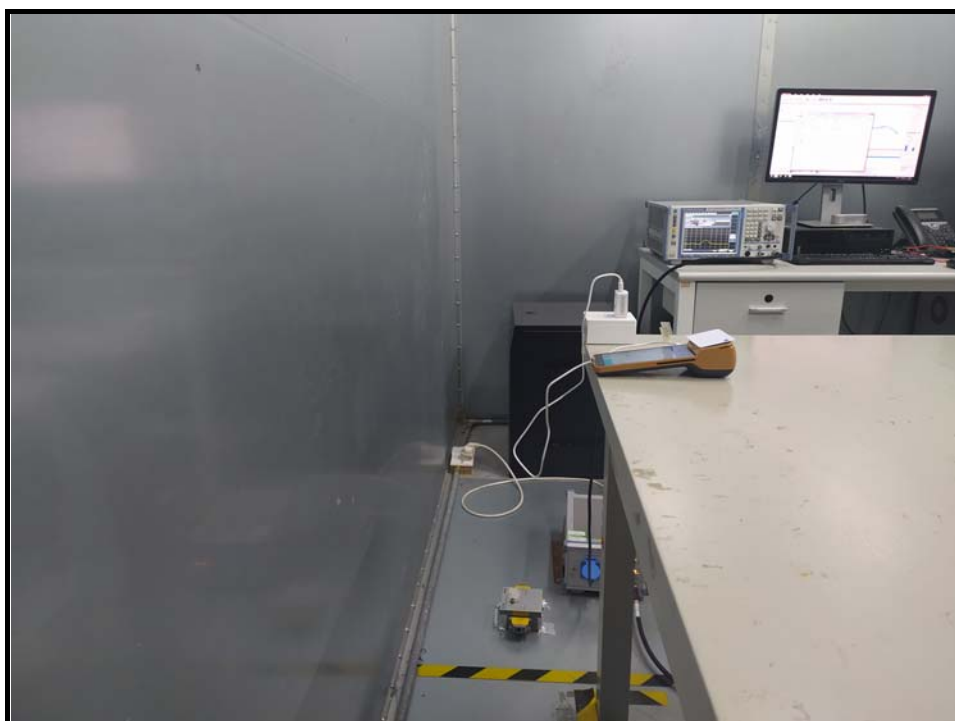
Fig. 4 Power line conducted emission setup photo
