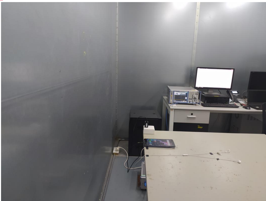
Fig. 3 Power line conducted emission setup photo
