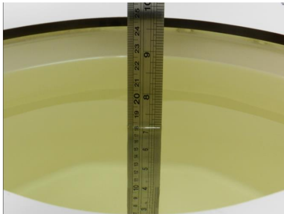
Fig 10.1 Photo of Liquid Height for Body SAR
