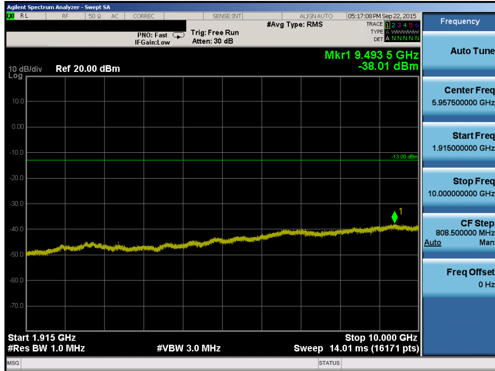
Plot 6-19. Conducted Spurious Plot (PCS CDMA Mode – Ch. 1175)
