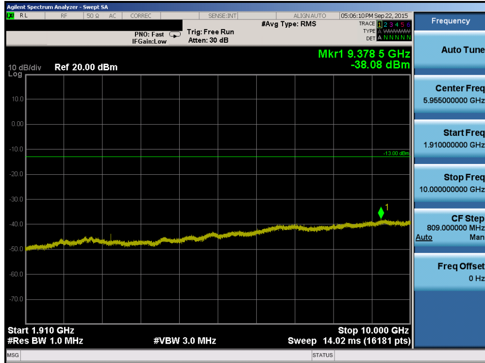
Plot 6-13. Conducted Spurious Plot (PCS CDMA Mode – Ch. 25)
