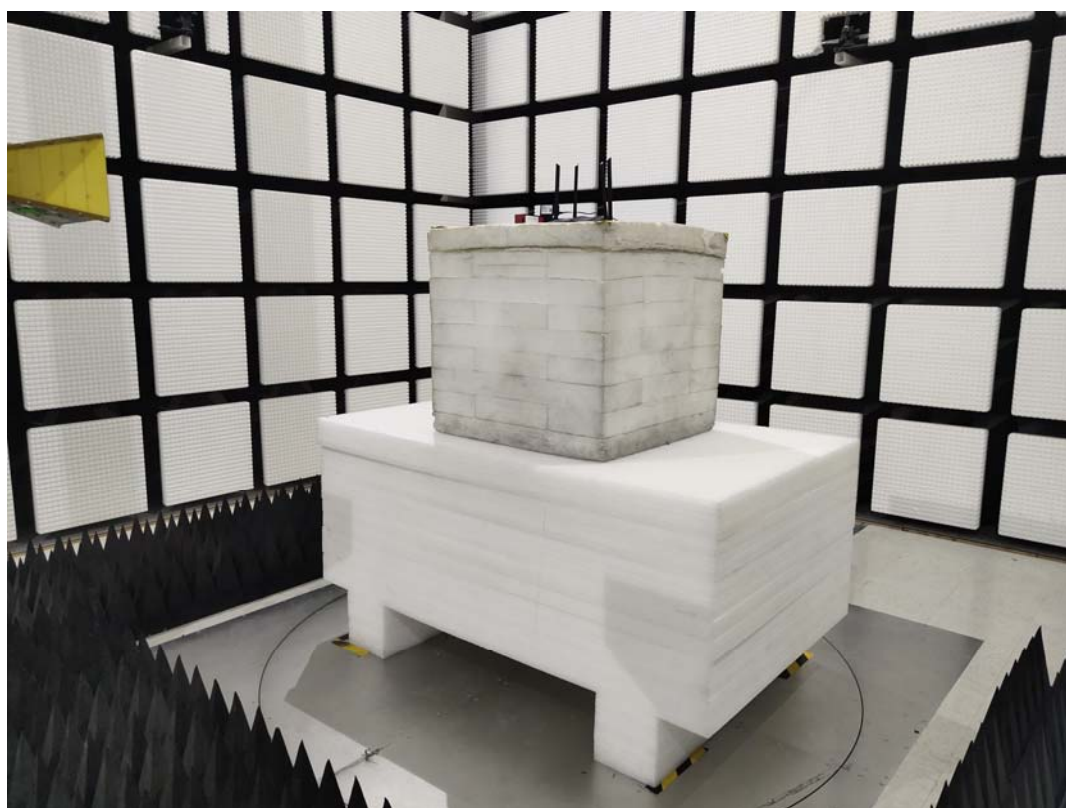
Radiated Emission Above 1GHz View
