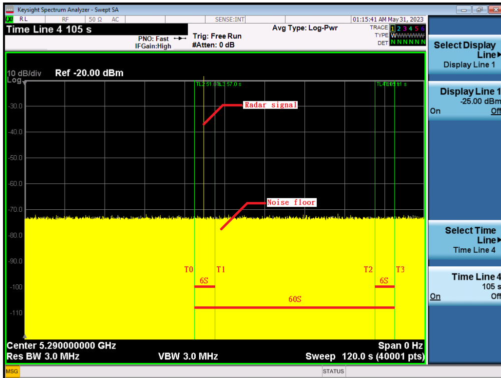
Radar Burst at the End of the Channel Availability Check Time
