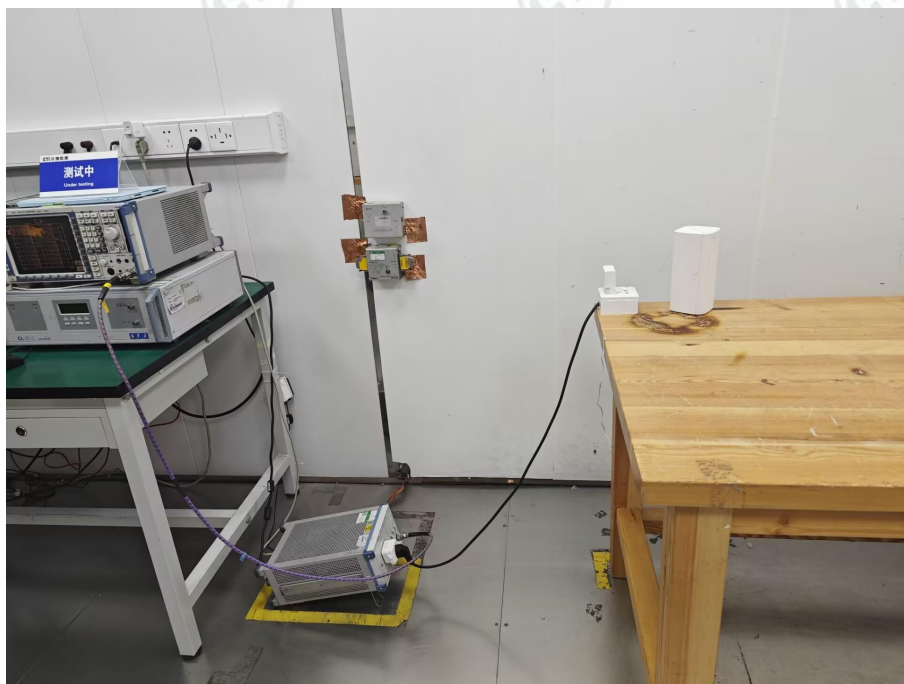
Conducted Emissions Test Setup
