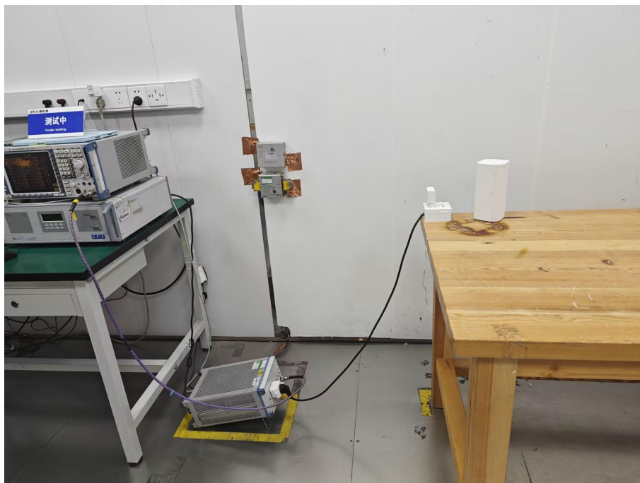
Conducted Emissions Test Setup
