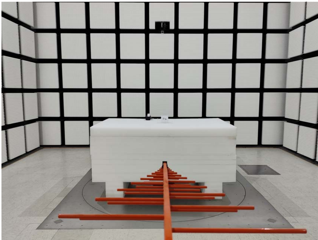
Radiated Emission Above 1GHz View
