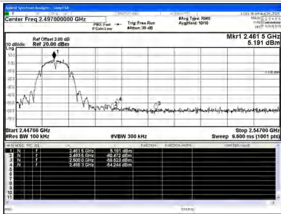
Band Edge NVNT b 2462MHz Ant1 Emission
