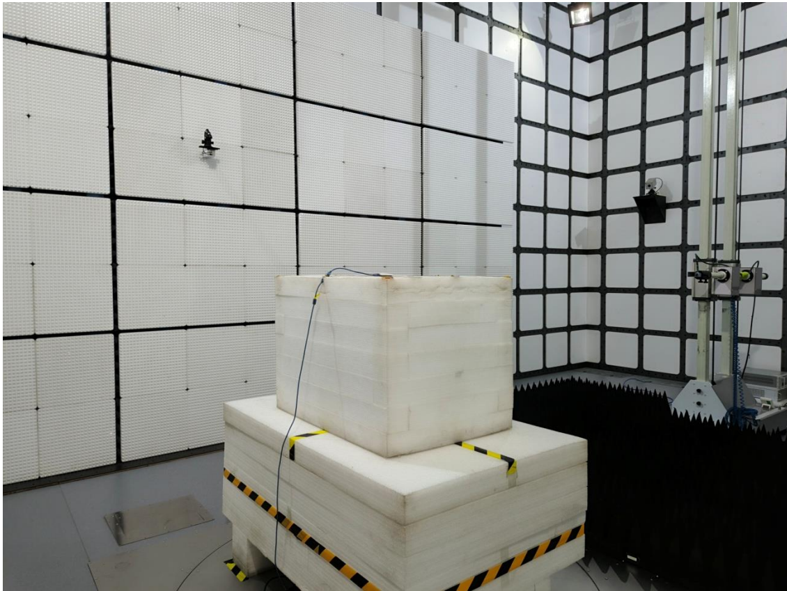
Radiated Emission 26.5-40GHz View
