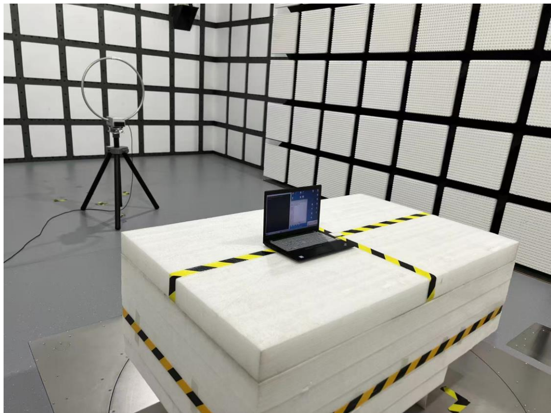
Radiated Emission 9 kHz-30 MHz Parallel View
