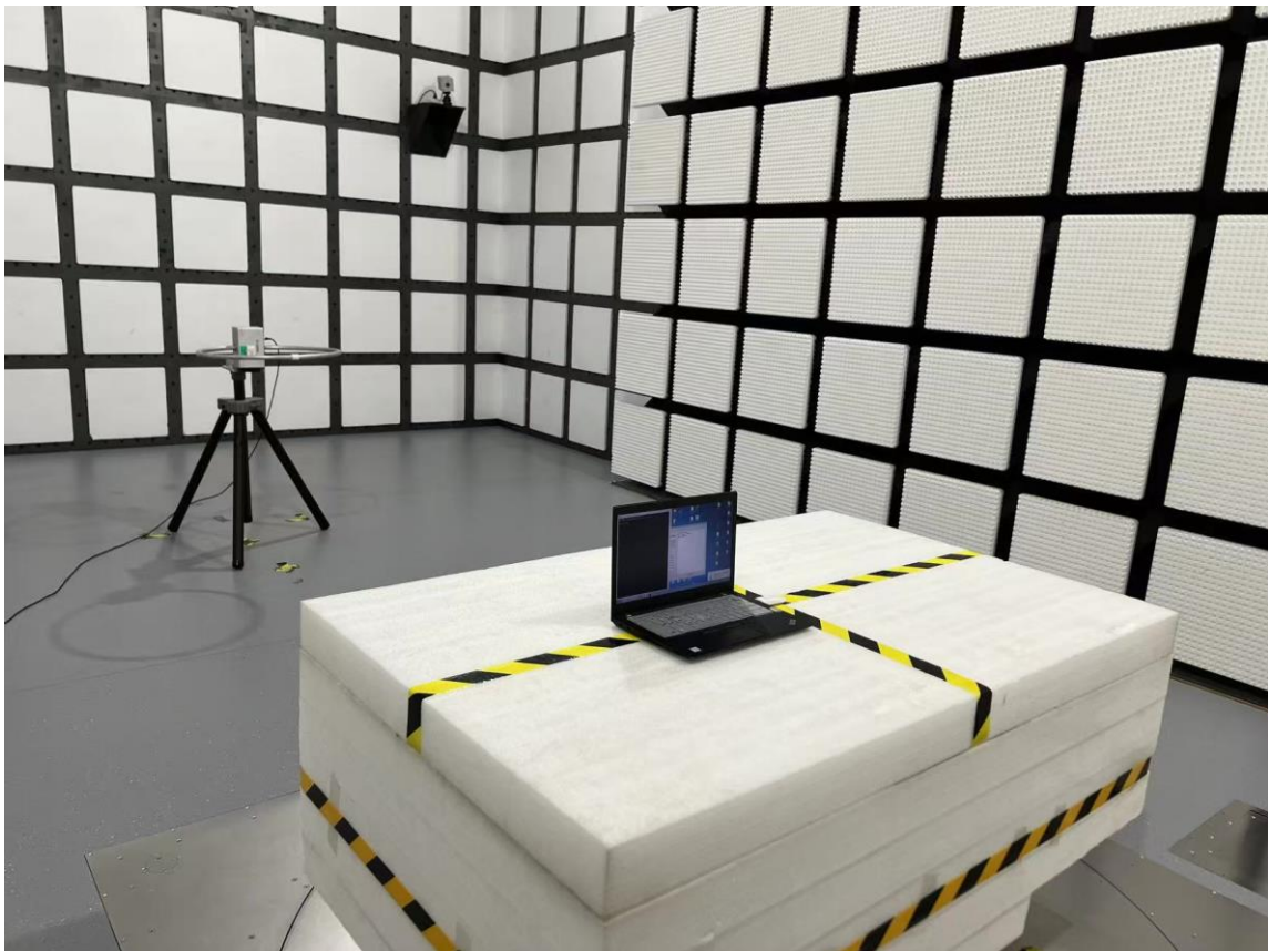
Radiated Emission 9 kHz-30 MHz Ground-parallel View
