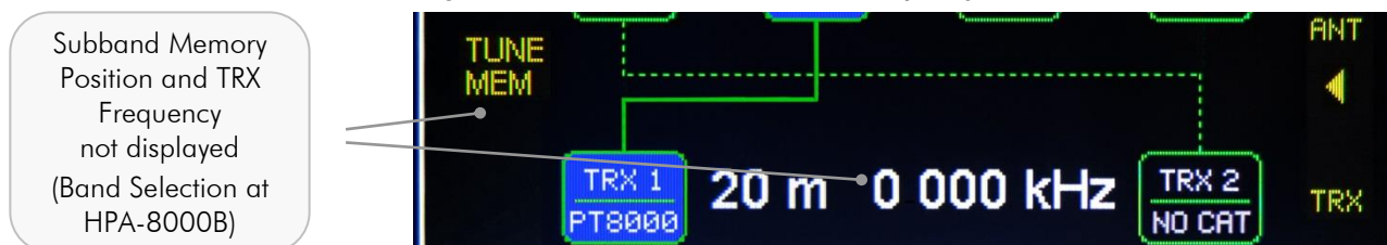
Fig. 8-6: Antenna Tuner activated – no Frequency Information
