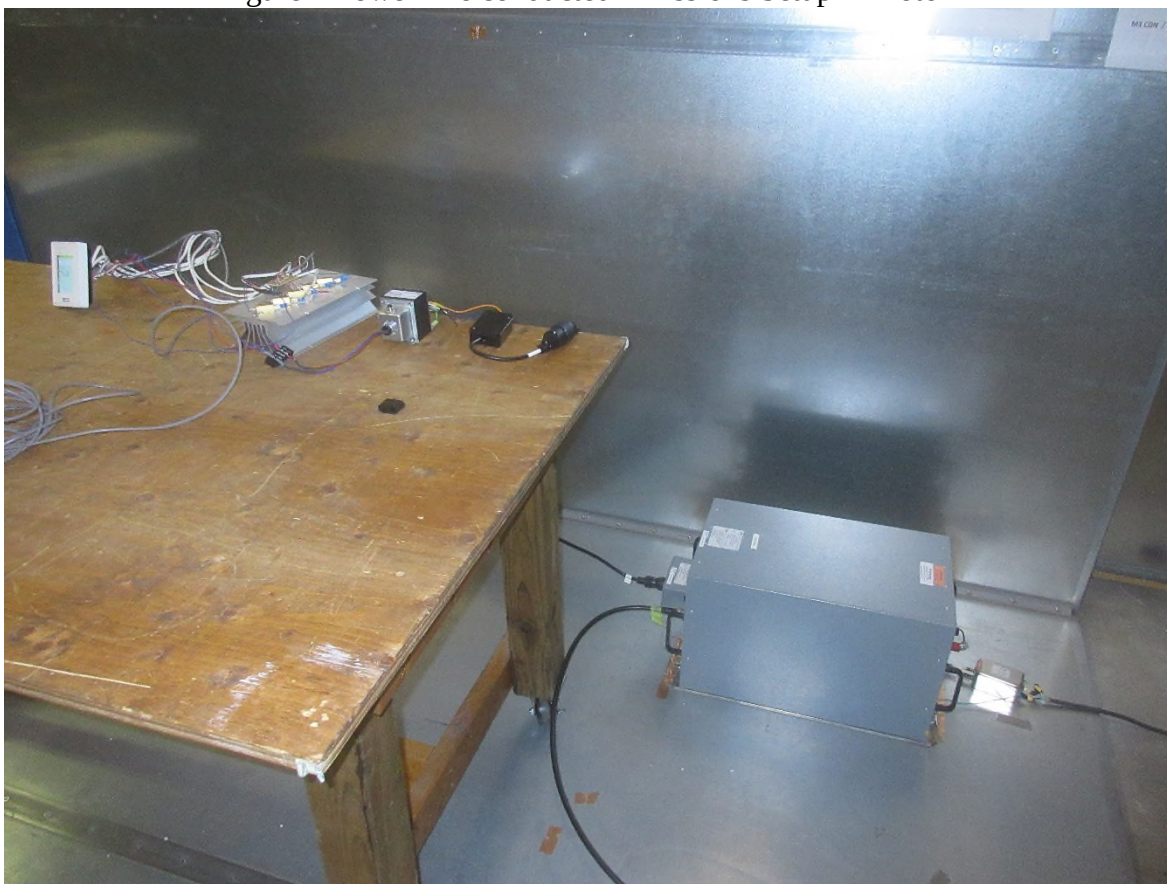
Figure 1 Power line conducted Emissions Setup – Photo 1
