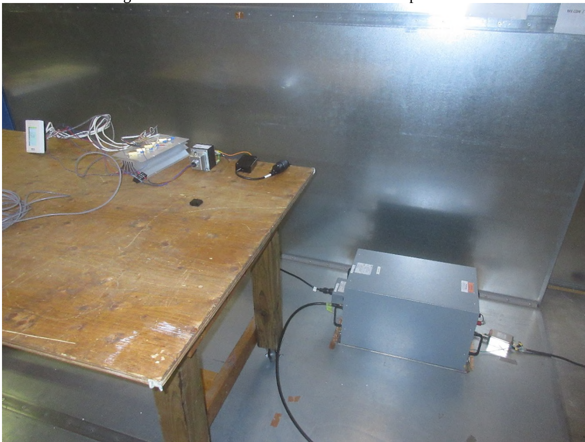
Figure 1 Power line conducted Emissions Setup – Photo 1
