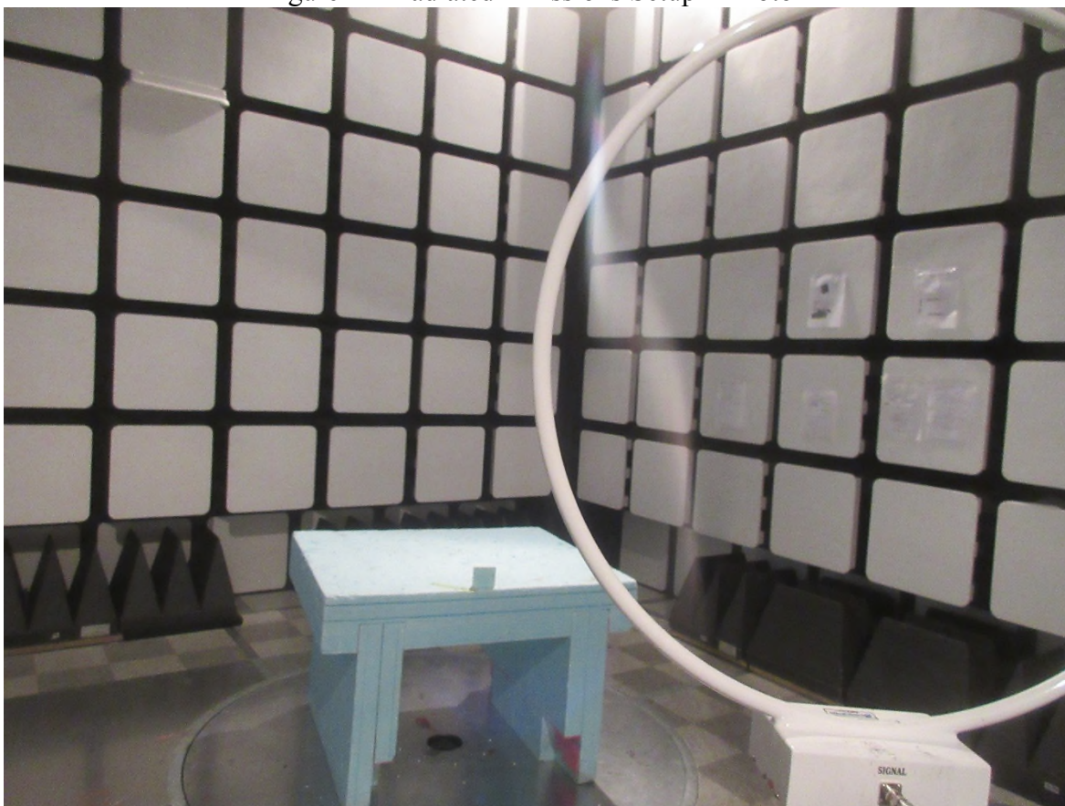
Figure 1 – Radiated Emissions Setup – Photo 1
