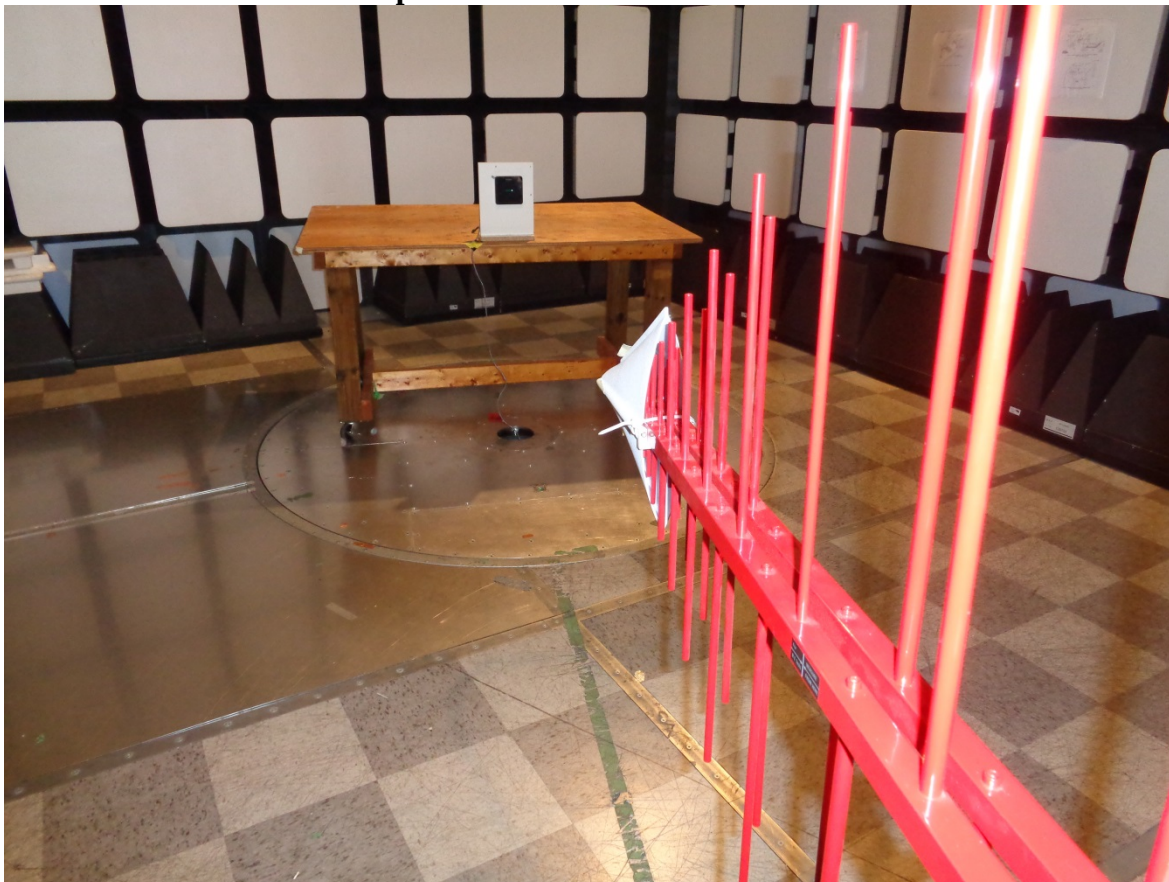
Radiated Emission Test Setup Photo #2:
