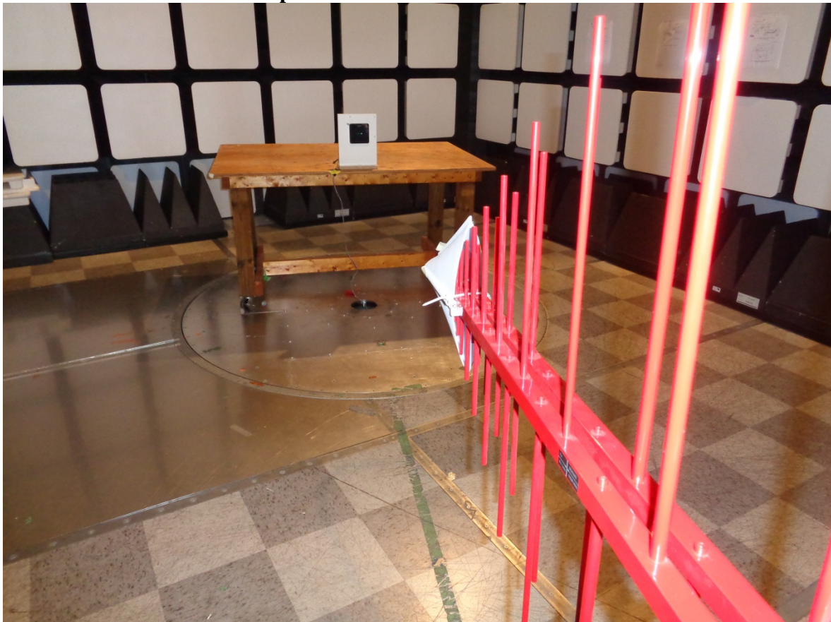
Radiated Emission Test Setup Photo #2:
