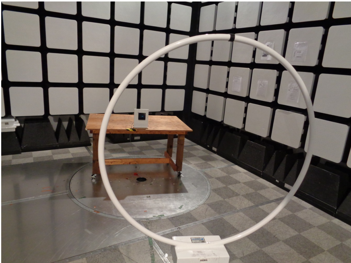
Radiated Emission Test Setup Photo #1:
