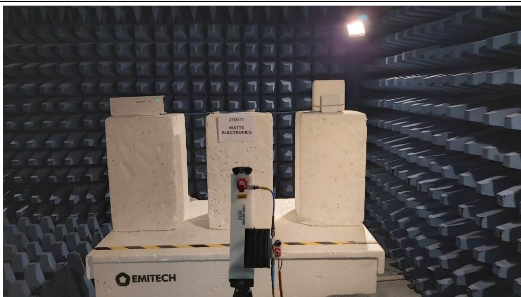
TEST SETUP PHOTO(S) - RADIATED MEASUREMENT / 18GHZ TO 26.5GHZ
