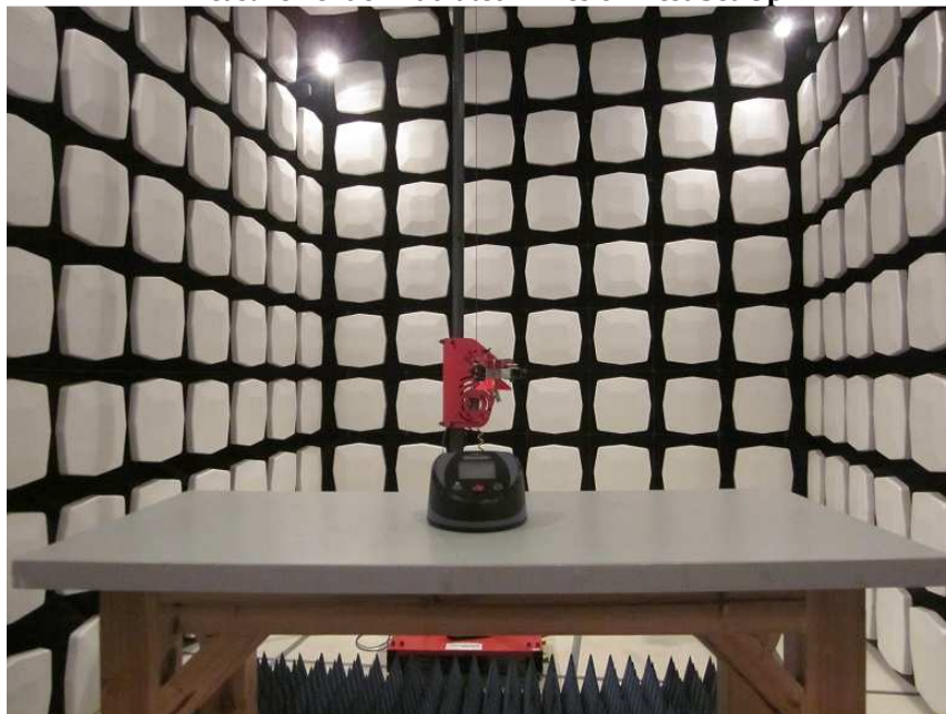
Measurement of Radiated Emission Test Set Up
