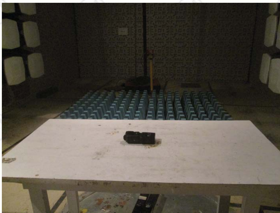
TEST SETUP OF RADIATED EMISSION (Above1GHz)
