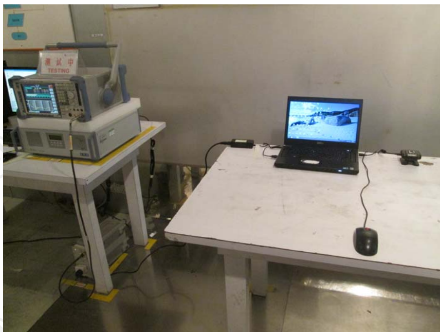
TEST SETUP OF CONDUCTED EMISSION
