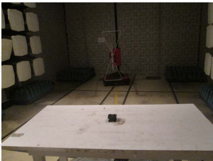
TEST SETUP OF RADIATED EMISSION (30MHz~1GHz)
